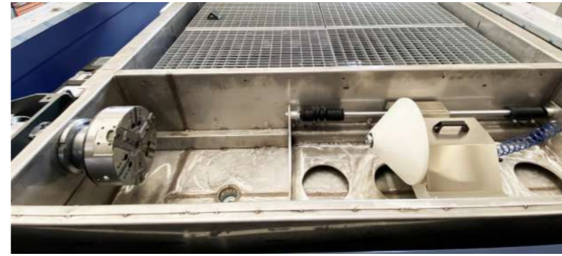
Tubocut • Motorized and CNC controller Mandrel with 3 connection clamps with manual clamping capability • Minimum diameter of the pipe: 64 mm • Maximum diameter of the pipe: 260 mm • Maximum length of the pipe: 1.000 mm • Maximum thickness of the pipe: 45 mm
